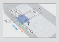
The software offers a design aid for the calculation of the load distribution through anchor brackets and determines the most critical load position.
